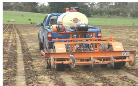
A hydro air seeder being used to sow native grass floret seed into a chemically fallowed paddock.
