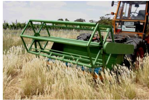
A reel-over-brush harvester gathering local provenance Austrodanthonia seed on the Henschke property in preparation for seeding their Hill of Grace vineyard.
