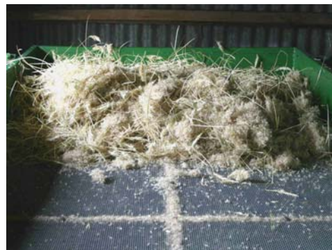
Harvested seed and stalks about to be separated with a vibrating 2x1-metre 3mm mesh sieve.
